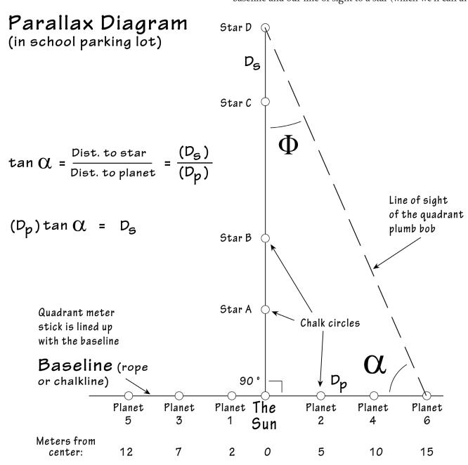
pha,  $\alpha$ ), the length of the opposite side ( $D_s$ ) divided by the adjacent side (baseline length or  $D_p$ ) is equal to the tangent function of alpha.
