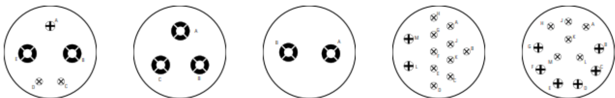
Figure 2-5: MIL-DTL-22992 contact configurations produced by MILNEC [14]
