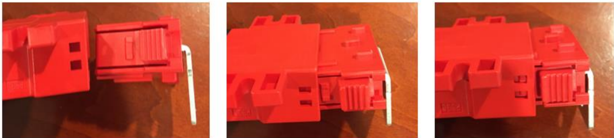
Figure 2-37: The Hirose PS3C connector with a spring-loaded clip
