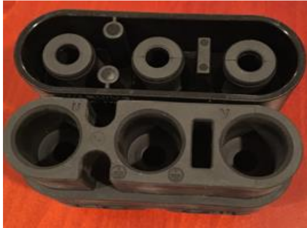
Figure 2-43: RobiFix connector, an example of soft-on-hard insulation waterproofing
