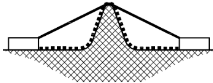
Figure 5-1: Creepage distance in the dotted line illustrated in UL 840 [67]
