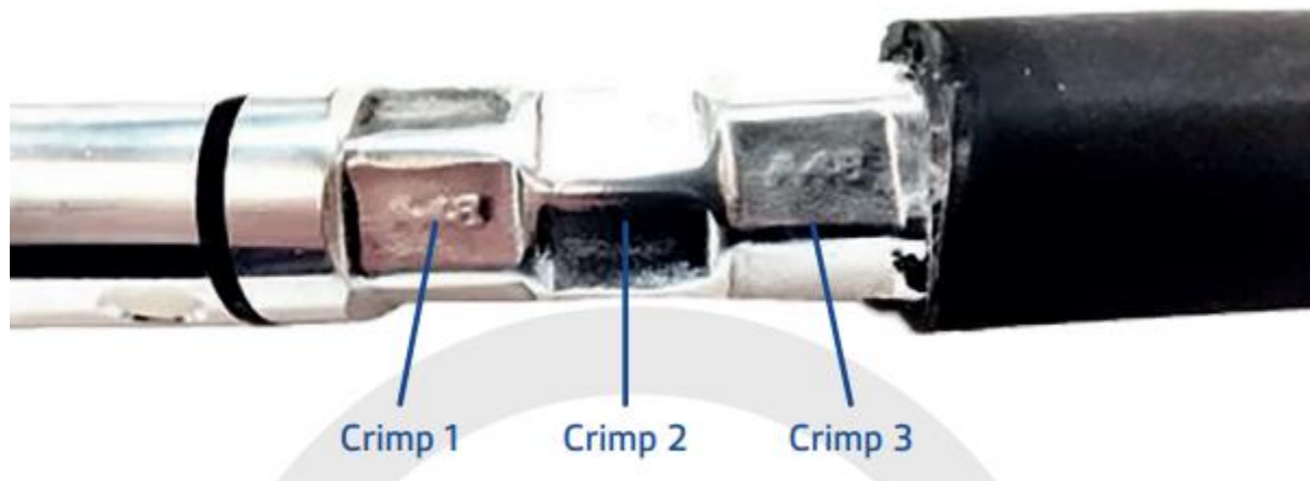
Figure 2-1: Multiple crimps made on a wire and Phase 3 connector using a hydraulic crimping tool and hexagonal die [11]
