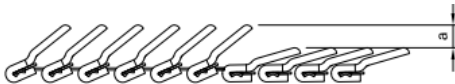
Figure 2-14: Two-component torsion louvers, half in compression [10]
