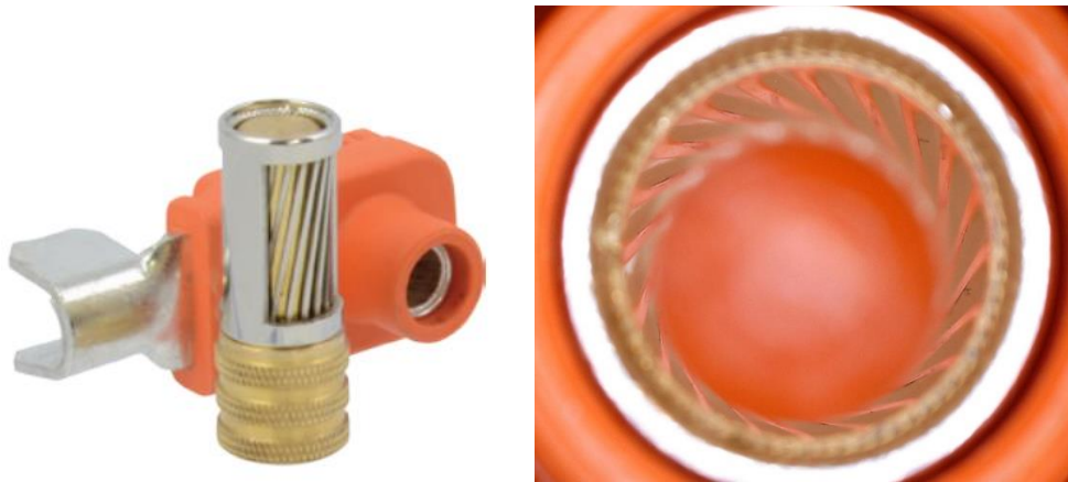
Figure 2-13: The hyperboloid technique called Radsok by Amphenol employed on the Radlok [18]
