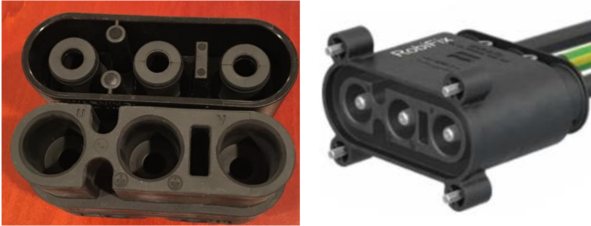
Figure 7-6: Concentric cylinder concept on the RobiFix by Stäubli [94]
