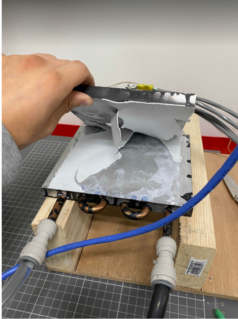
Fig. 7. Image showing the breakdown of silicon based TIMs after being under compression and heat loads. This break down causes difficulty in clean up and is an undesirable performance trait for a TIM being used for the iPEBB.
