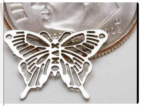
This butterfly pattern was generated in 0.02-inch-thick stainless steel while testing of one of the company's smallest abrasive waterjet nozzles. The part also shows how once a program is developed, it can be scaled to other sizes. As shown here, the butterfly's wingspan is 0.40 inch, but the pattern could be enlarged to fit an 8-by-10 foot sheet of metal, if so desired.
