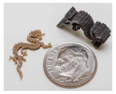
Abrasive waterjet can cut a variety of workpiece materials, including metal, rubber, glass, stone and composites. These materials can be difficult to machine conventionally. For example, the tan dragon shape (left) is made from 2.4-mm-thick fiberglass material. The black dragon is made of carbon epoxy.
