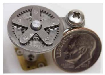
This is the assembled gear set. This assembly shows that waterjet cutting could be used for producing internal components for small clocks or pocket watches. Benefits include faster programming and cutting than conventional machining methods. This assembly also represents the value of this process in prototyping. Parts for a complete assembly can be produced quickly and cost effectively.
