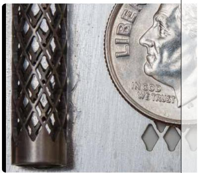
Made from a titanium tube, this mesh cage is an orthopedic surgical implant for human bone repair. The "unfolded" pattern to the right under the coin shows how a 2D pattern can be transferred onto a cylindrical part. A rotary axis was used to cut the pattern into the tube with one of its smallest machine nozzles.
