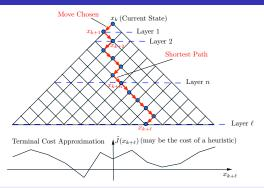
We obtain a trajectory  $\{x_k, x_{k+1}, \dots, x_{k+\ell}\}$  that minimizes the shortest distance from  $x_k$  to  $x_{k+\ell}$  PLUS  $\tilde{J}(x_{k+\ell})$ . We then use the first move  $x_k \to x_{k+1}$ .
