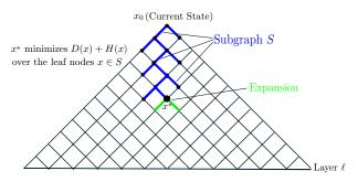
We use a less regular graph, which is expanded at each iteration based on a shortest path computation
