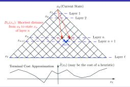
• The "forward" DP algorithm: The shortest distances  $D_{n+1}(x_{n+1})$  to layer n+1 states are obtained from the shortest distances  $D_n(x_n)$  to layer n states as follows:
