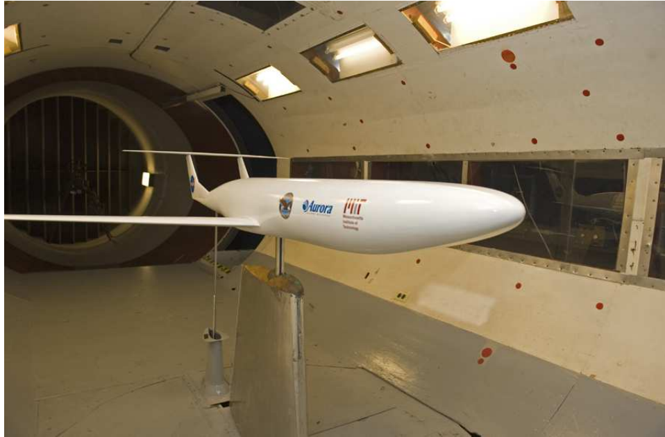
Figure 14. 20:1 scale low-speed wind tunnel model.
