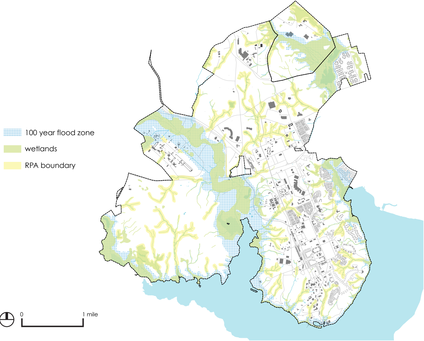
Figure 54. Water Resources. The airfield and Humphrey's Engineering Center are areas of concern being located in the flood zone. (Source: Fort Belvoir DPW, 2014 Fort Belvoir DEIS, and Fairfax County)
