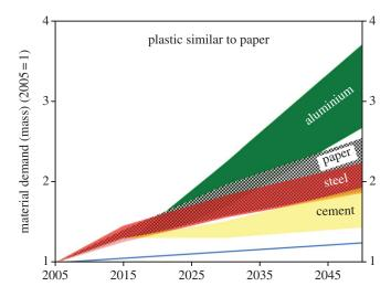
**Figure 8.** The range of future demand for aluminium, paper, steel, plastic and cement constructed from forecasts provided by the IEA [7]. Plastics demand projection adapted from Allwood *et al.* [5]. The bottom curve (blue) leading to 1.25 in 2050 shows the maximum demand allowed in order to meet the goal of halving the world's energy use by materials with a 56% improvement in energy intensity (see text).
