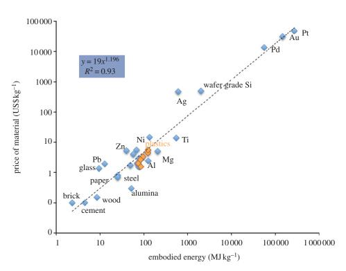
**Figure 6.** Price of various materials plotted against the embodied energy of the materials. The data for embodied energy comes from Ashby [10], for material prices for metals from the *Mineral yearbooks* [17], plastics from IDES [28] and brick, wood and glass from Ashby [10]. Plastic prices are for year 2011, and all others are for 2009.
