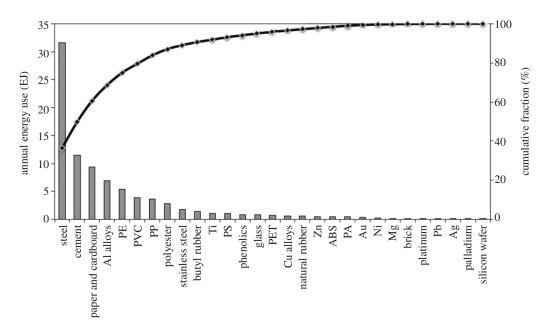
**Figure 1.** Annual primary energy used for the production of 29 materials worldwide, cumulative scale on the right. PE, polyethylene; PVC, polyvinyl chloride; PP, polypropylene; PS, polystyrene; PET, polyethylene terephthalate; ABS, acrylonitrile butadiene styrene; PA, polyamides. Adapted from Ashby [10].
