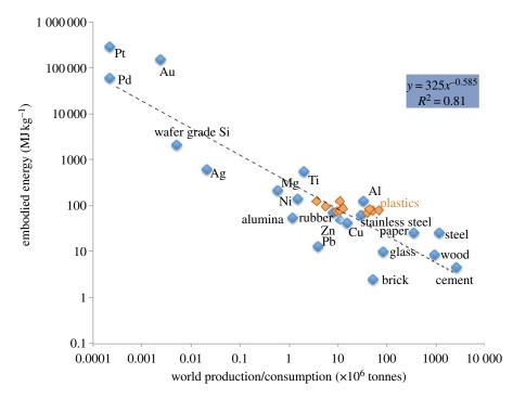
Figure 7. Energy intensity e versus world production Q for various materials of construction. Adapted from Ashby [10].
