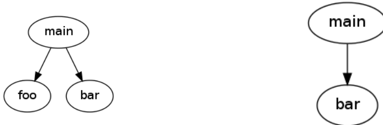
Figure 5-2: CFGs that demonstrate imprecisions in flow-sensitive code in static analysis (left) and dynamic analysis (right)
