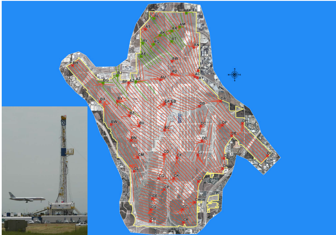
Figure 2-3 Horizontal drilling allows the exploitation of the Barnett reservoir below the Dallas/Fort Worth (DFW) Airport (Star Telegram 2015)
