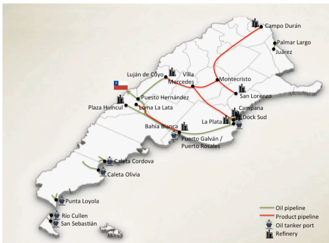
Figure 2-17 Crude oil and product main pipelines in Argentina in 2015 (Author with data from ASoE)
