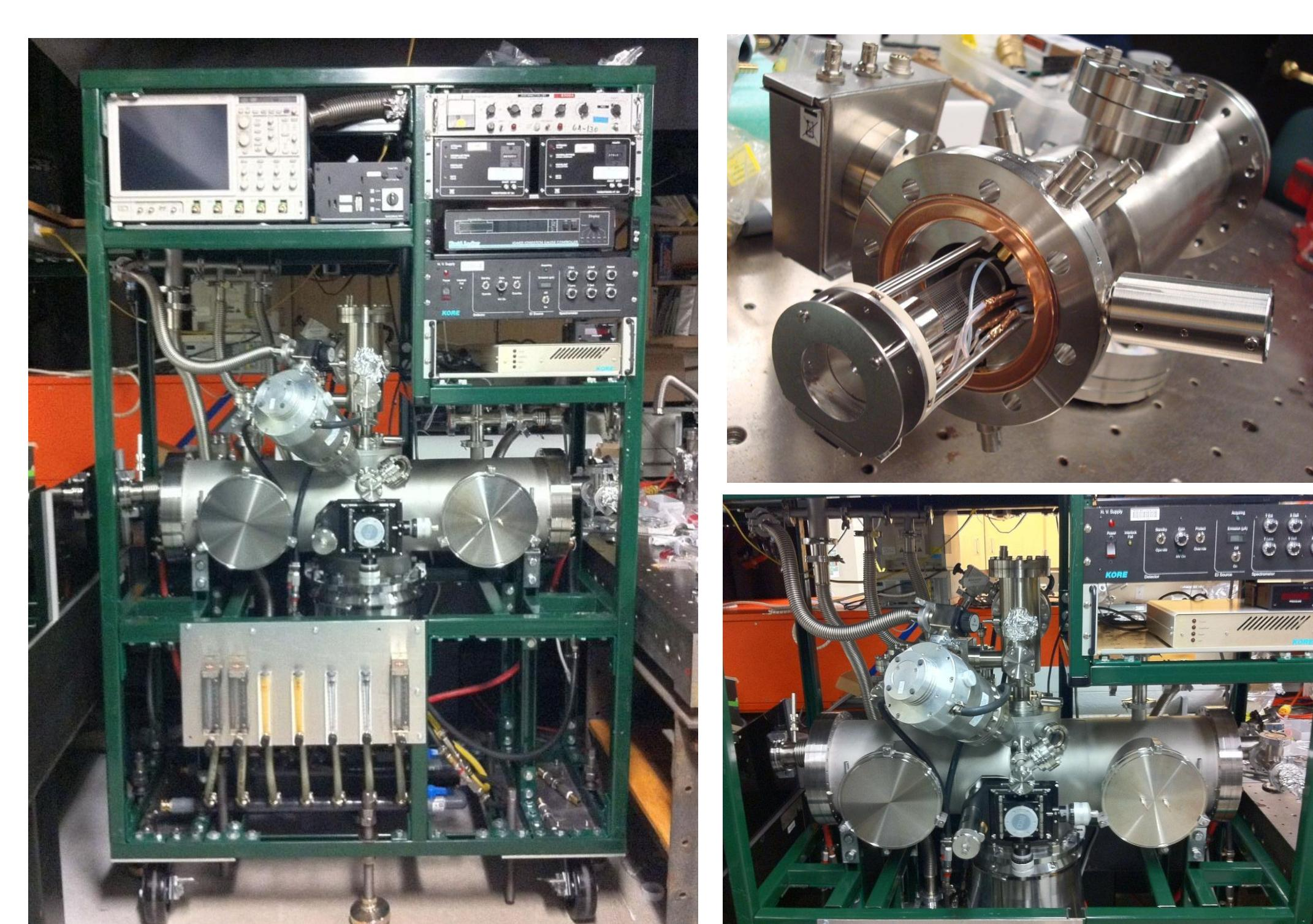
The Kore TOF-MS (top right) is shown mounted on the chamber (bot. right), which has been mounted to a custom cart along with all of the associated electronics (left).
