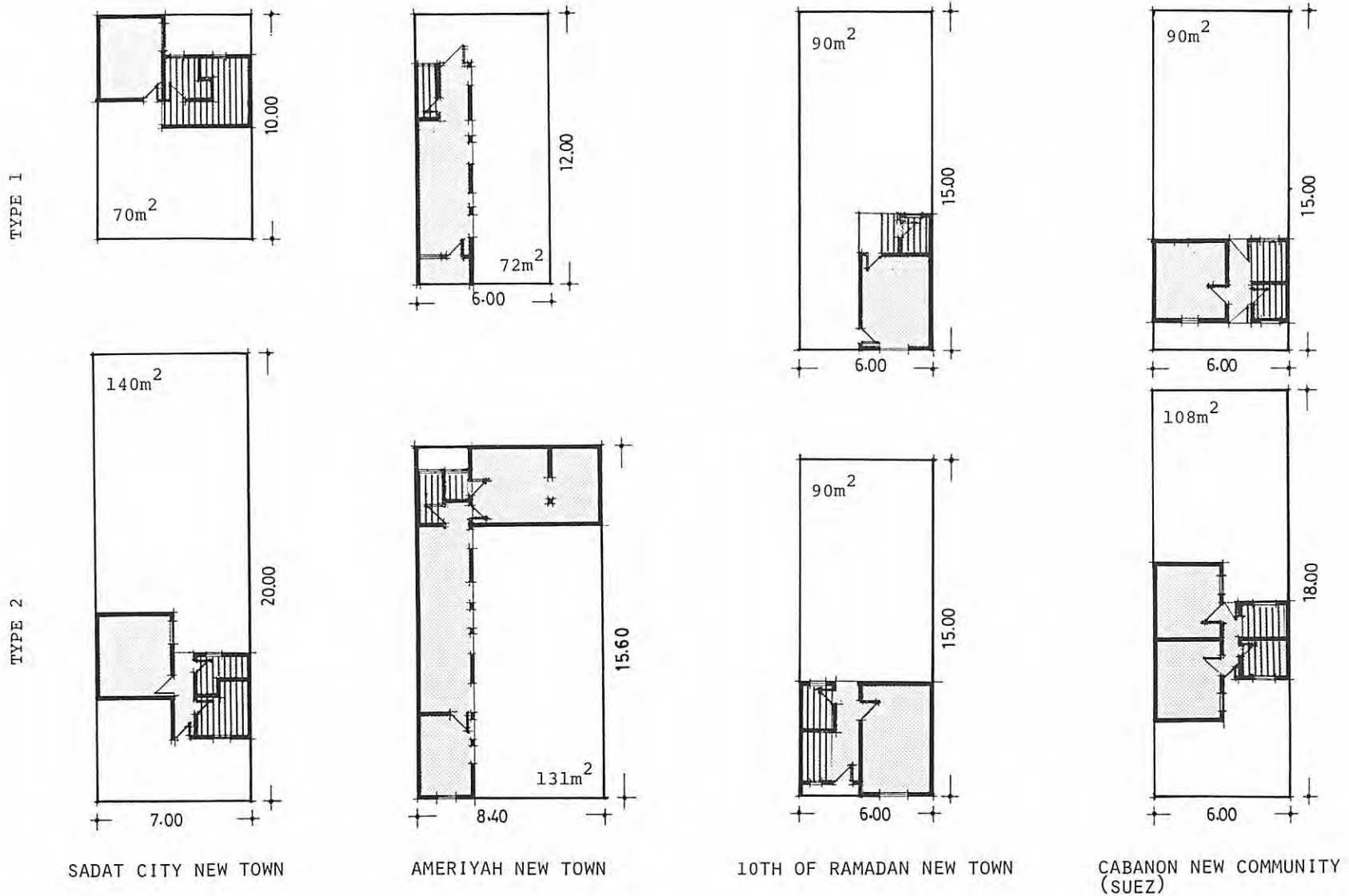
Figure 3: LOCATION OF THE CORE ON THE PLOT AND NUMBER OF INITIALLY BUILT ROOMS
