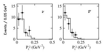
FIG. 3. Transverse momentum distributions for data (crosses) and Monte Carlo (solid line) for neutrino events (left) and antineutrino events (right) with a wrong-sign muon. A LNV signal would appear as an excess of events in the antineutrino mode.
