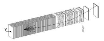
FIG. 1. Schematic of the NuTeV detector, showing the calorimeter and the toroid spectrometer.
