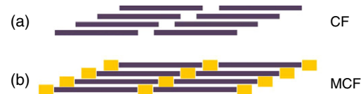
Figure 2. Overview of the two structures considered here; subplot (a) shows a CF and subplot (b) shows an MCF. The structures are loading in uniaxial tension along the axis of the TC molecules.
