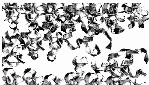
Fig. 11. Crack propagation creates a round fracture surface due to local refolding of the protein during crack motion. Observation of such detail in fracture behavior is only possible using atomistic simulation. Bonds within a protein do not break, only bonds between different protein molecules that are columbic, H-bonds or dispersive vdW interactions.
