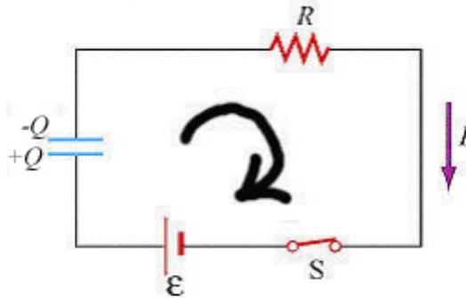
Figure 1: Choices for current, circulation, and charge on capacitor
