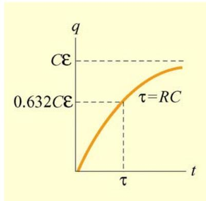
Figure 7: charge vs. time graph
