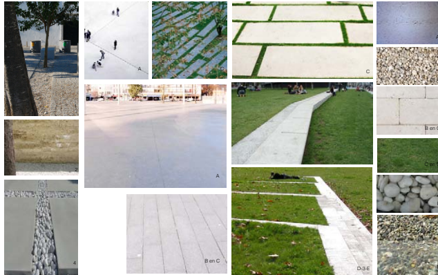
10. Perspective and references showing the selected gradient from impervious to pervious material in the courtyard
