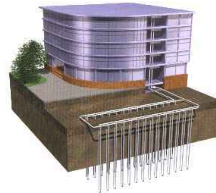
Figure 11-16 Cut-away section of a closed loop vertical system
