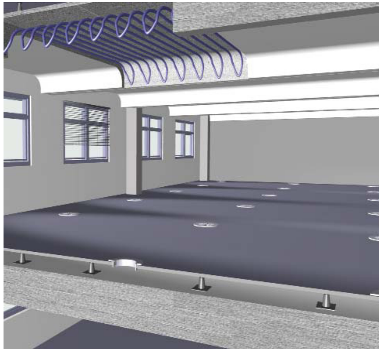
Figure 7-14 Cut away section of coils embedded in slab
