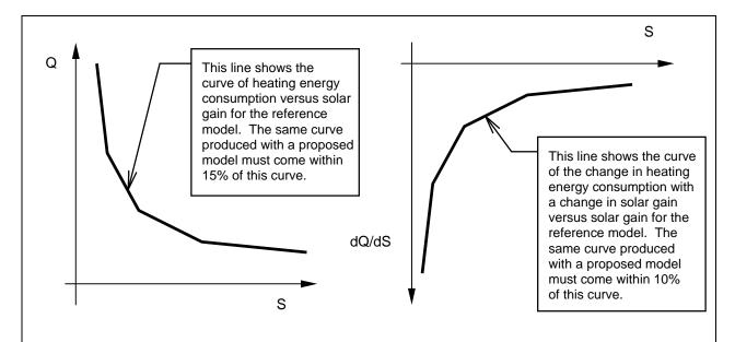
**Figure 7-1.** To be accepted as a compliance model the proposed model must predict heating energy consumption (Q) and changes in heating energy consumption (dQ) to within a certain percentage of the same predictions made with a reference model. Shown for example are what might be typical plots versus solar gain. Similar plots would have to made for Q and dQ versus other parameters of interest, e.g. *RSI-value*, thermal mass, infiltration rate.
