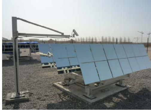
Figure 2 Typical ganged type heliostat and tracking sensor. The sensor arm and heliostat azimuth axis are aligned on a common radial line extending from the tower axis, which is to the left.
