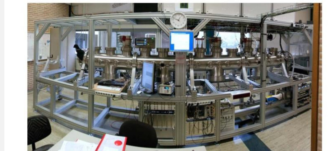
A panoramic picture of the four meter long traveling-wave decelerator that has been built in Groningen. It is in use for decelerating packets of the heavy diatomic molecule SrF, which is a prototypical system for the investigation of broken symmetries.
