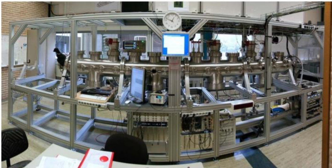
A panoramic picture of the four meter long traveling-wave decelerator that has been built in Groningen. It is in use for decelerating packets of the heavy diatomic molecule SrF, which is a prototypical system for the investigation of broken symmetries.
