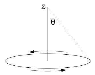
Take the ring to have radius R, and consider a current of magnitude I circulating as shown. What is the magnitude and direction of the current a point z above the ring's center? Set up Biot-Savart:
