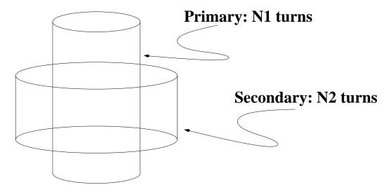
The idea is that we drive a time varying current through the primary, making a time varying magnetic flux:
