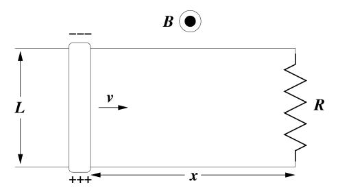
The changing flux in this case is due to the continually changing area. We get an EMF whose magnitude is  $\mathcal{E} = BLv/c$ , and that (by Lenz's law) drives a current which circulates counterclockwise in the loop.
