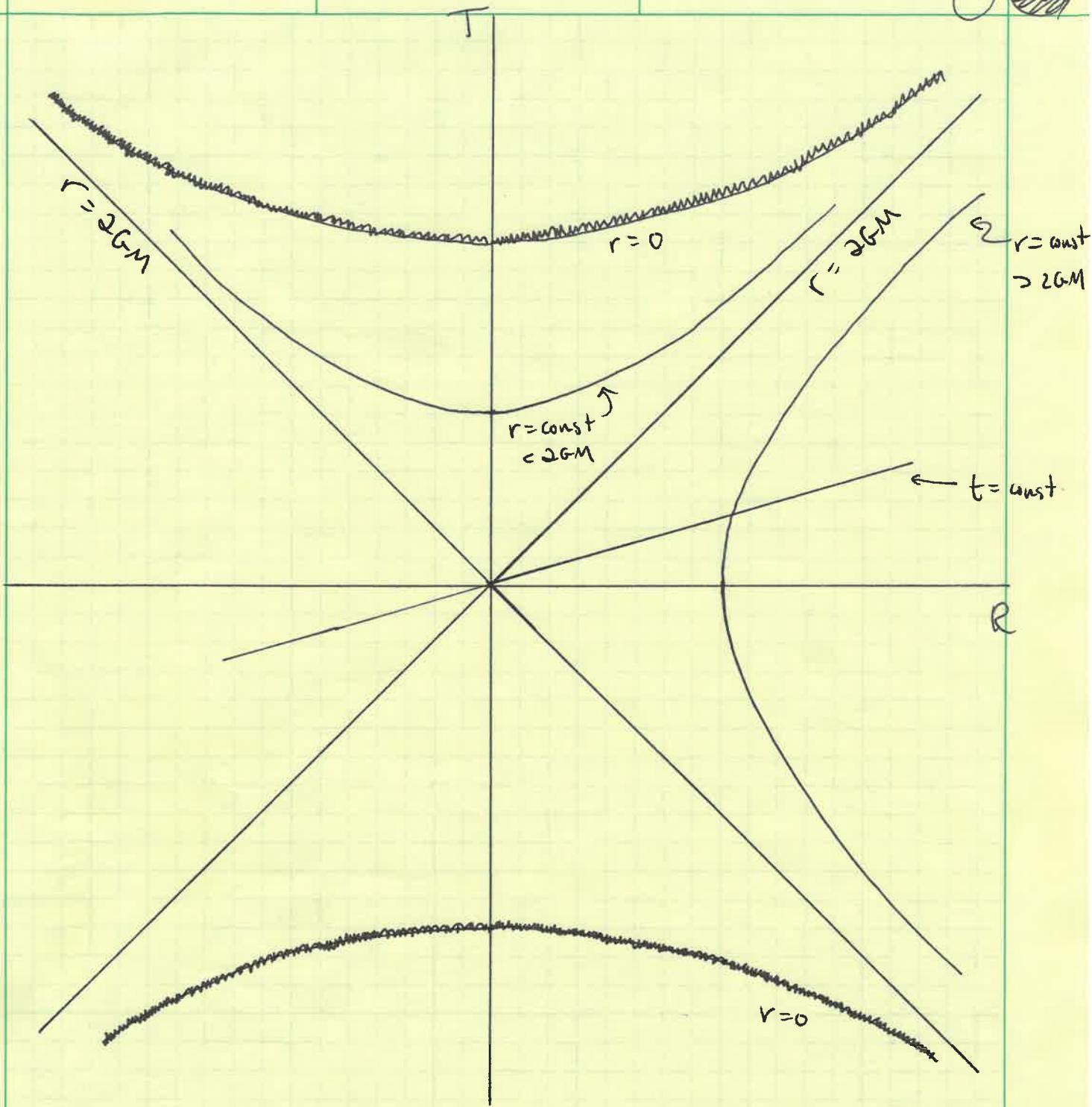
Since speed of light trajectories are  $45^\circ$  lines on this diagram, clear that no physical trajectory can move from  $r < 2GM$  to  $r > 2GM$ . Interior is "causally disconnected".
