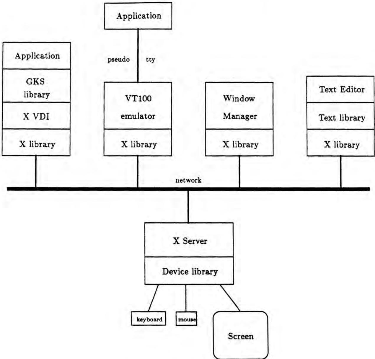
Figure 1: System Structure
