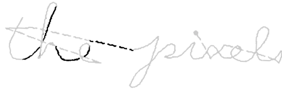
Figure 4-3: Calculation of the sgn(x-max(x)) bit for the word “the” only. The highlighted portions are encoded with 1 and the gray portions are encoded with 0 , for the sgn(x-max(x)) bit.
