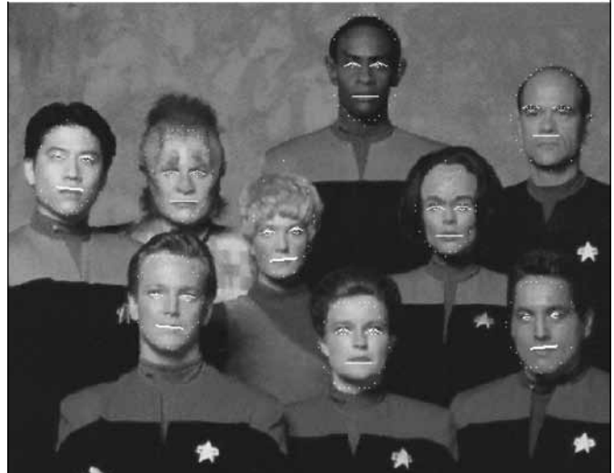
Figure 4. Example of face detection and facial feature extraction. (Image courtesy of Hankyu Moon and colleagues, IEEE Trans. Image Processing , Nov. 2002, pp. 1209-1227.)
