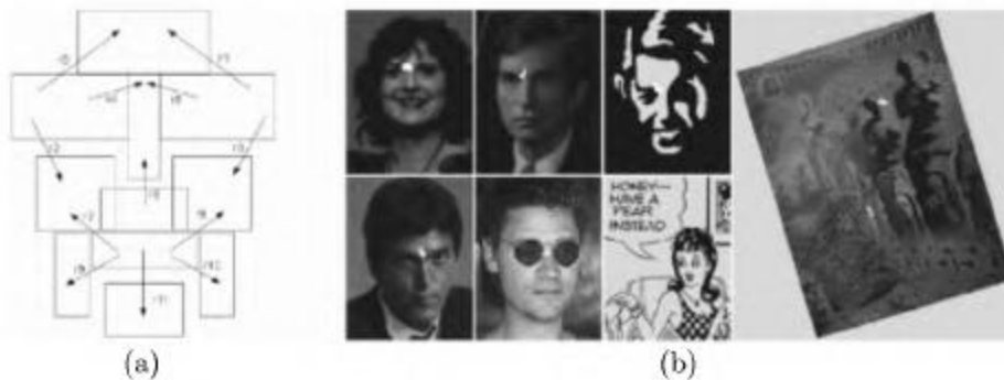
Figure 8: A small collection of ordinal relations (a), though insufficient for high fidelity reconstruction, is very effective for pattern classification despite significant appearance variations. (b) Results of using a local ordinal relationship based template to detect face patterns. The program places white dots at the centers of patches classified as faces. (From Thoresz and Sinha, in preparation.)
