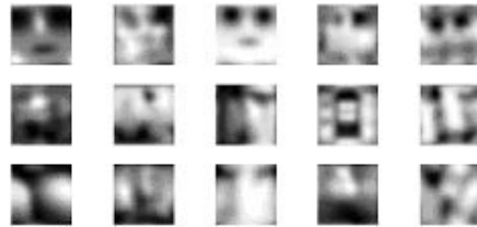
Fig. 2. A few of the non-face patterns used in our experiments. The patterns comprise false alarms of a computational face-detection system and images with similar spectra as face images.
