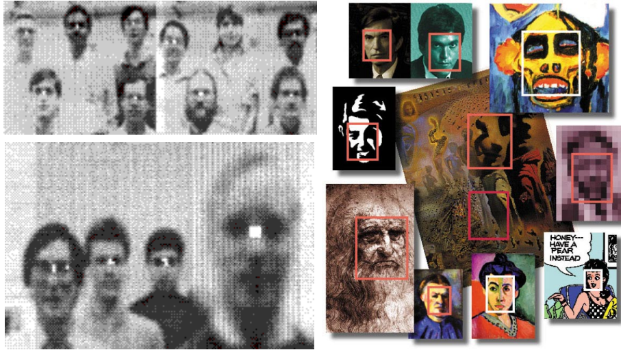
Fig. 9. Testing the face-detection scheme on real images. The program places a small white square at the center of, or a rectangle around, each face it detects. The results demonstrate the scheme's robustness to varying identity, facial hair, skin tone, eye-glasses and scale.
