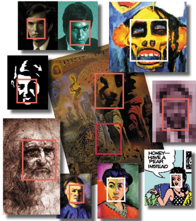
Figure 8. Results of using a qualitative representation scheme to encode and detect faces in images. Each box corresponds to an image fragment that the system believes is a face. The representation scheme is able to tolerate wide appearance and resolution variations.
