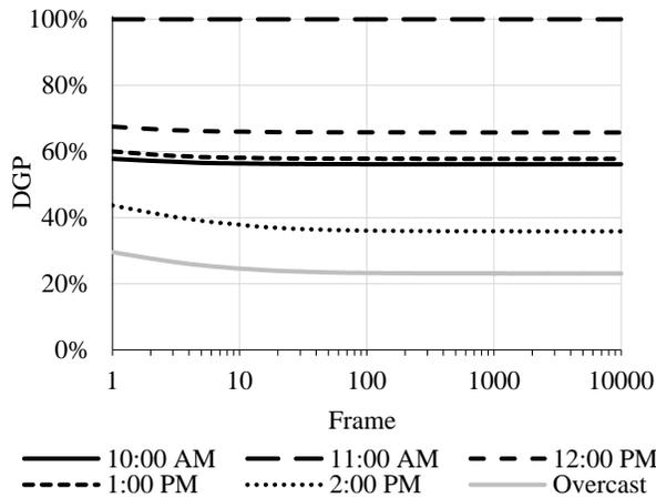
Figure 6: DGP for the scenes in Figure 5 converges downward as rendering progresses. Greater values undergo less change.
