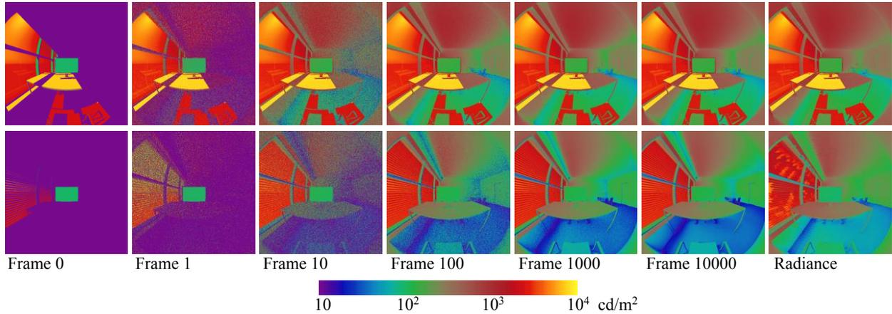
Figure 2: Falsecolor renderings of an office with unshaded windows (top) and venetian blinds (bottom) show a progression from direct contribution only (frame 0) to well-sampled diffuse contribution (frame 10000). Comparison to RADIANCE rendering (right) shows the accuracy of our method.
