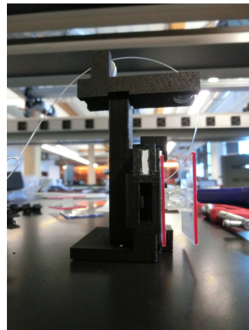
FIGURE 3.5 3D printed shear test structure with piece
