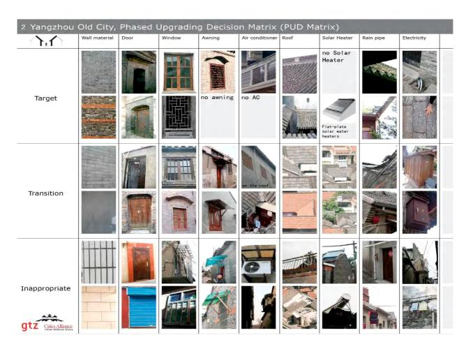
Fig. 7 The 'Phased Upgrading Decision Matrix' – Facade Level Source: GTZ Project Team
