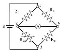
**Solution:** When there is no current flowing through the ammeter, the potential difference V(b) - V(a) = 0. Therefore V(c) - V(a) = V(c) - V(b). If we assign currents as shown in the figure below then  $V(c) - V(a) = I_1 R_1$  and  $V(c) - V(b) = I_2 R_2$ .
