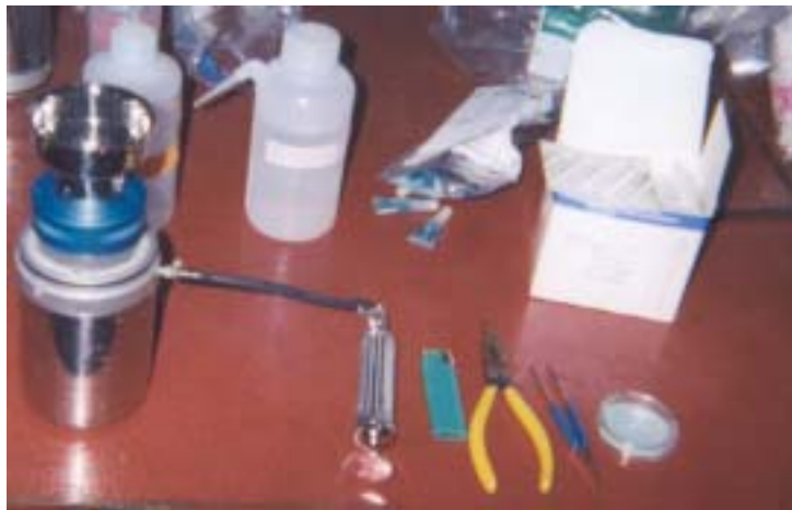
Figure 4.8 Millipore portable membrane filtration assembly (left) with vacuum hand pump, lighter, pliers, forceps, petri dish, 0.45 \mu m filter paper, m-ColiBlue24 TM nutrient broth ampules and sterilized water.
