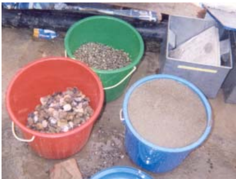
Figure 4.7 Filter media: clockwise from left, gravel, coarse sand and fine sand.
