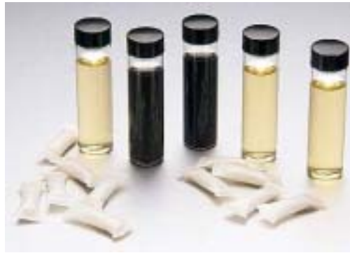
Figure 3.1 H 2 S test vials and powdered media packets. Vials with black precipitate indicate presence of H 2 S producing bacteria (HACH, 2003).
