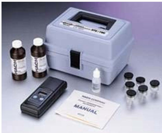
Figure 4.10 Turbidimeter field kit. Counter-clockwise from left: calibration standards, pocket turbidimeter, instruction manual and sample vials (HACH, 2003).
