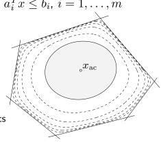
inner and outer ellipsoids from analytic center:
