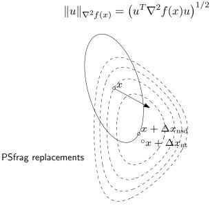
dashed lines are contour lines of f; ellipse is  $\{x+v\mid v^T\nabla^2 f(x)v=1\}$  arrow shows  $-\nabla f(x)$
