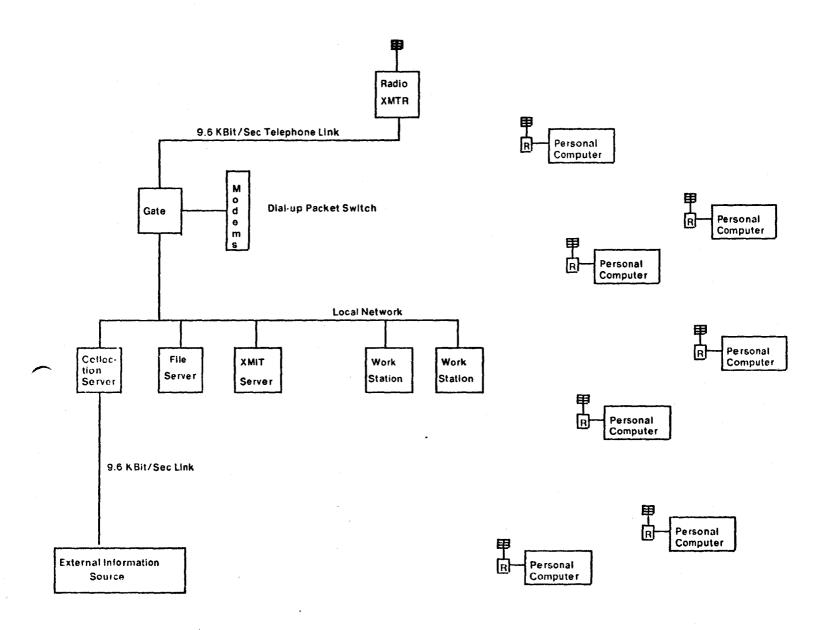
Figure 11-1: Base System Block Diagram
